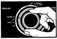
**B.** Stop on a number in the cycle you want. The numbers are minutes of wash time. The drawing shows 6 minutes of agitation in the REGULAR NORMAL Cycle.
